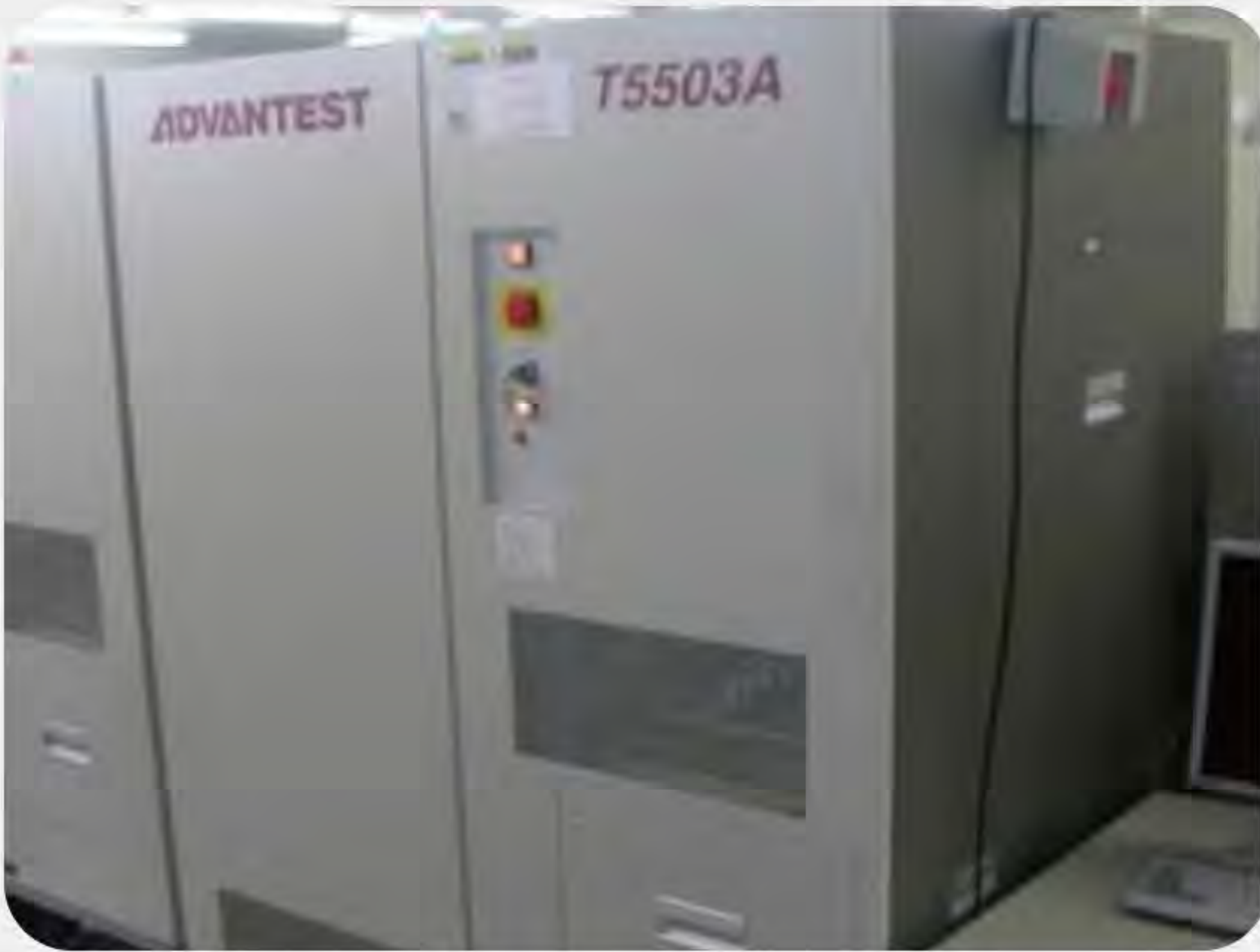
Wide-Temp. IC Sorting via Automatic Test Equipment (ATE)
